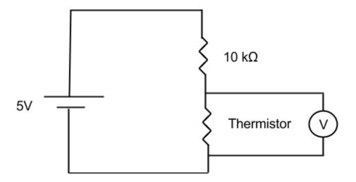
This means that the numbers that you are seeing on the screen are related to the **voltage across the thermistor**. We would expect a voltage of 0 - 5 V depending on the resistance, however because the NXT cannot use decimals it gives us a range of 0-1023. With this information we have the following relationship.
